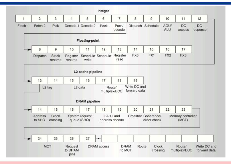
Fetch/decode 3 inst/cycle, 3 integer units, 3 address units 3 FPU/multimedia units, 2 load/stores to D-cache/cycle
