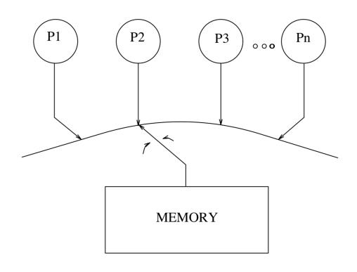
simple memory system: no caches, no write buffers
