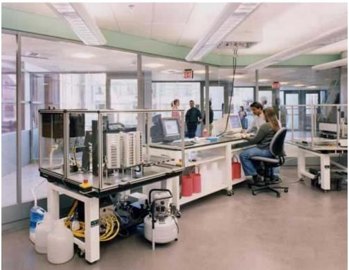
Glass interior walls permit natural lighting to flow into the work areas, creating an open environment that facilitates collaboration. All utilities are supplied by overhead service modules and casework is provided in two-foot-wide modular units.
