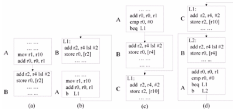
Fig. 1. Different Branch Cost of Different Edges in Control-Flow Graph
