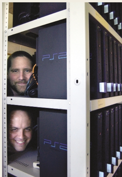
Mike Showerman [top] and Craig Steffen pose with the supercomputer cluster they built from Sony Playstation 2 consoles.
