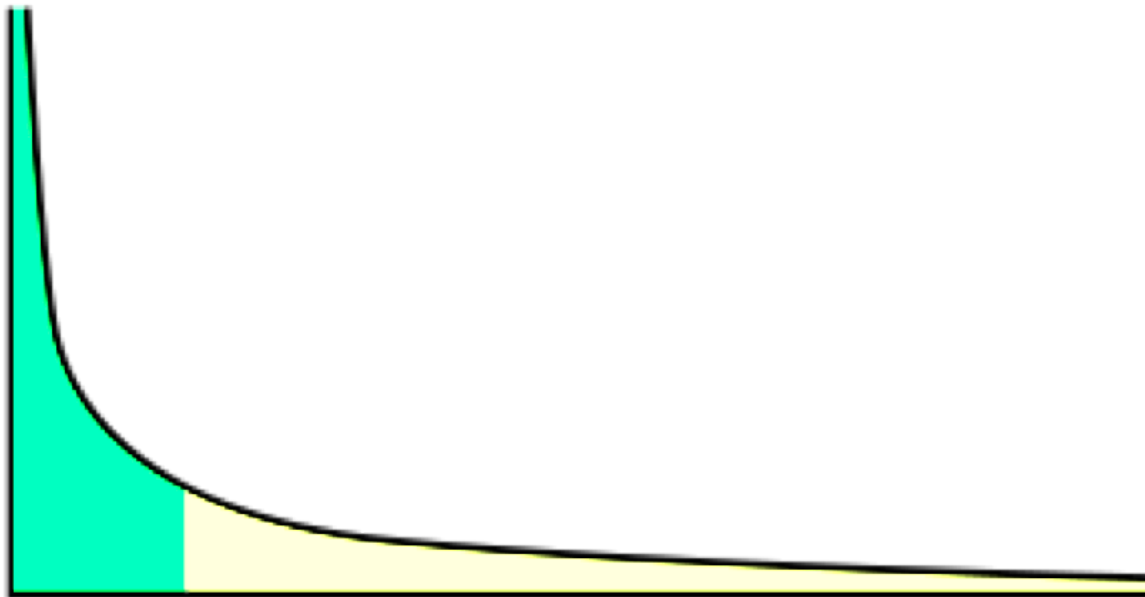
Figure 1: Power law. Suppose we sort the weights of elements in our stream. For the heavy hitters problem, we expect the distribution to fall off faster than x^{-k} for some power k . Here, x -axis shows elements, y axis is contribution/weight of the elements
