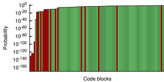
**Figure 12: P4wn’s probabilistic profiles are a useful guide for adversarial testing, as there is a strong correlation between a code block’s probability and the expensiveness of the processing behavior. (Top 110 code blocks out of 220 are shown.)**
