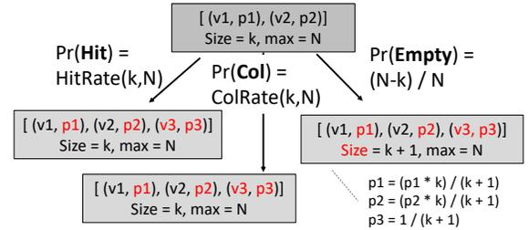
**Figure 5:** For each access to the probabilistic data store, P4wn forks three paths and updates the probabilities using the current state of the data store. A similar analysis is performed for sketches and Bloom filters.
