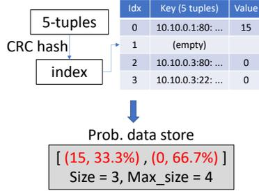
**Figure 4:** We create a probabilistic data store for each hash table, which encodes the distribution of all possible values in this greybox. This avoids the need for keeping track of a large symbolic state space and analyzing complex CRC functions, improving scalability.
