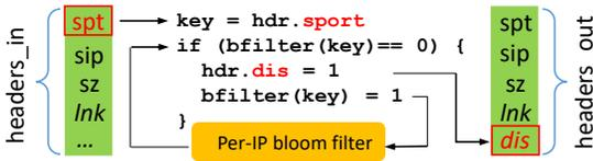
**zip** performs a join between two sets of headers using a common key. Internally, the compiler generates two sketches (or bloom filters), and a packet triggers two queries, one to each sketch. Consider ‘zip(sip,tot,cnt)’, which produces a total traffic volume and a packet count for each source IP:
