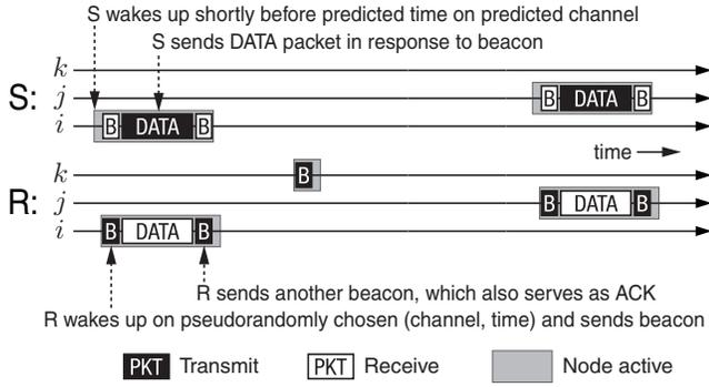
**Figure 1: Sender  $S$  sends data packets to receiver  $R$  using EM-MAC. Only three of the channels are shown here, labeled  $i$ ,  $j$ , and  $k$ . At the time of  $R$ 's second beacon, no node has a packet waiting to send to  $R$ .**
