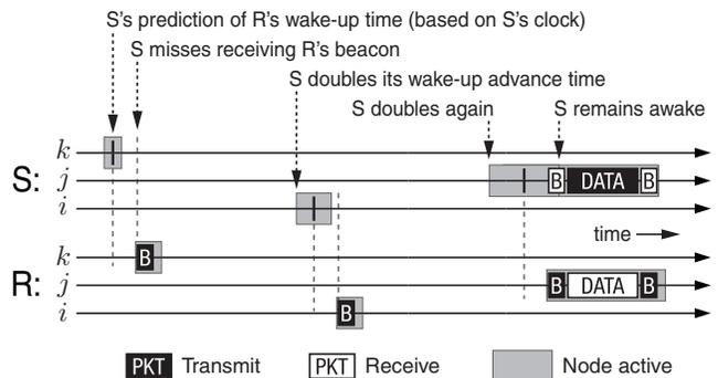
**Figure 2: Sender  $S$  and receiver  $R$  have a large time difference. To rendezvous with  $R$ ,  $S$  exponentially increases its wake-up advance time and the waiting time around the predicted receiver wake-up time, which quickly makes up for the time difference between  $S$  and  $R$ . Each wake-up time of  $R$  predicted by  $S$  is marked by a vertical bar during each active time of  $S$ .**
