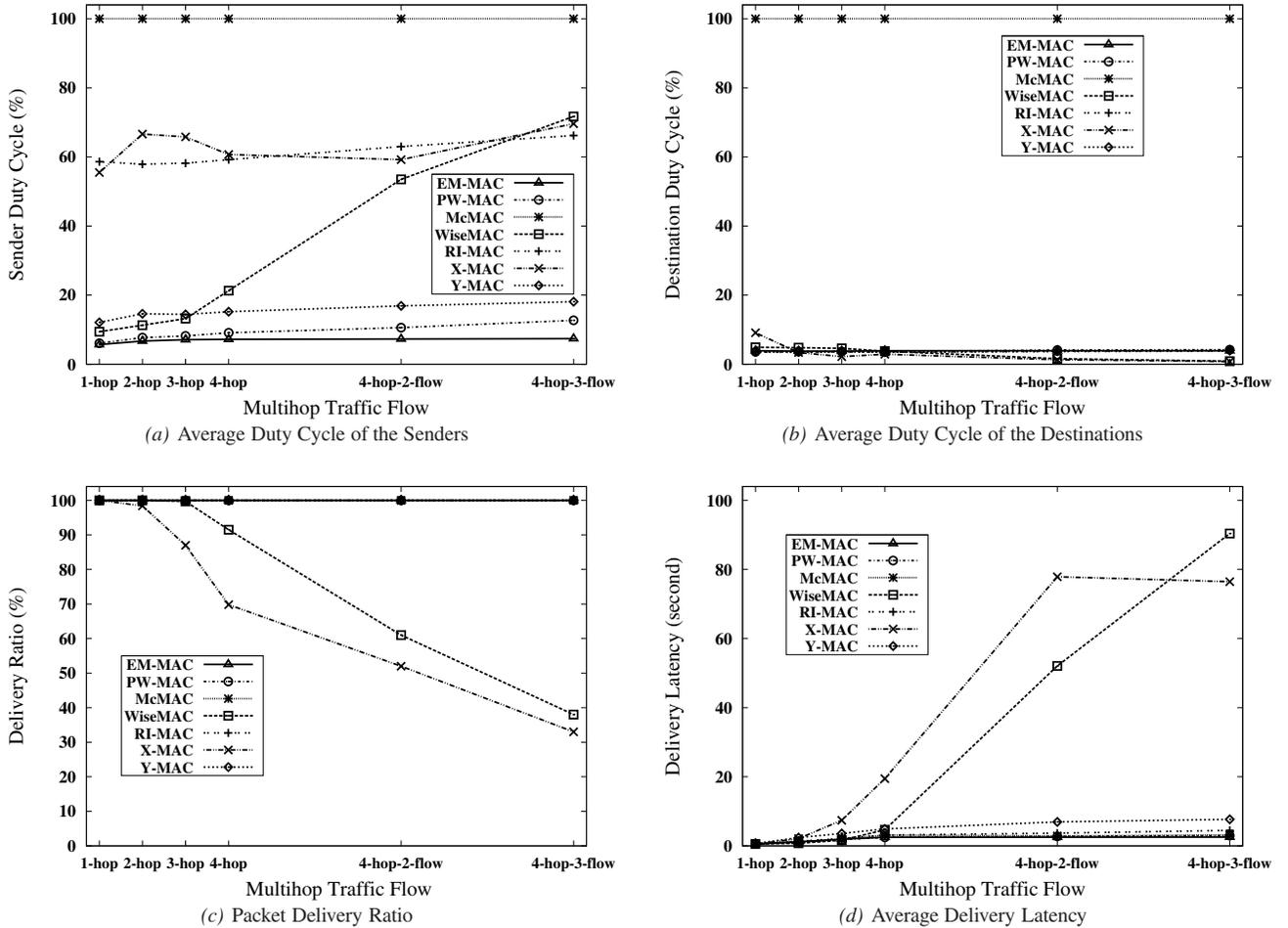
**Figure 4: Performance of EM-MAC, PW-MAC, McMAC, WiseMAC, RI-MAC, X-MAC and Y-MAC on a multihop MICAz testbed. The hop-length of the traffic flow varies from 1 to 4 and the number of 4-hop traffic flows ranges from 1 to 3.**
