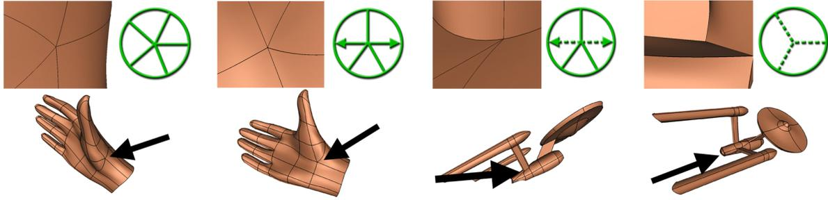
**Figure 4:** Four corner configurations arising during realistic modeling. The upper left pictures are close-ups of both the network and the lofted surface. The upper right diagram depicts the layout of the  $\psi_i$ . Dotted edges are creases. Pairs of arrows denote cross curves.
