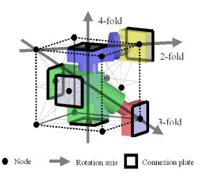
Fig. 1. Construction of a lattice module in space group F432 with face-centered cubic cell. The module has four bodies, six connectors and three actuators. The connection plates are in special position on the nodes and have 4-fold symmetry. The three actuators have 2-fold, 3-fold and 4-fold rotation axes corresponding to geometric elements of the space group, therefore this module has  $2 \times 3 \times 4 = 24$  discrete configurations.
