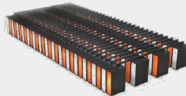
ExaScale Data Center Max of ~500 racks, 10's of MW, O(10^9) concurrency
