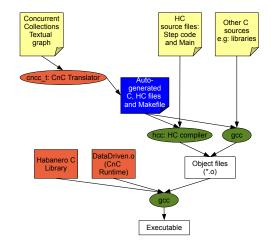
Figure 4. CnC-HC Implementation Flow
