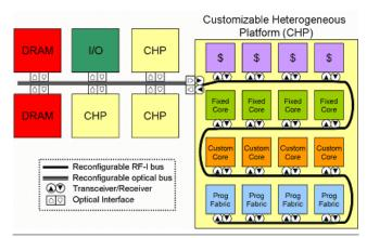
Figure 1. Customizable Heterogeneous Platform
