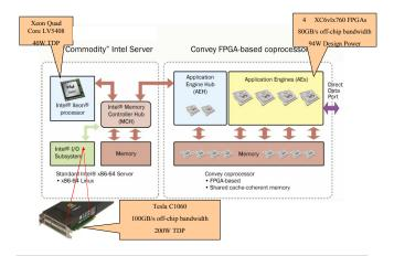
Figure 7. Diagram of the Convey HC-1ex Hybrid Computer
